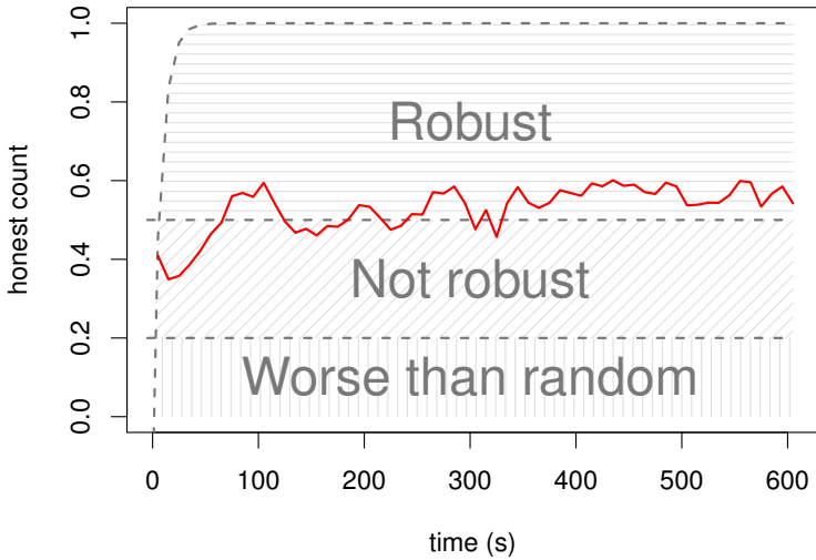
Figure 3.10: The number of honest nodes found by the measuring node over time (the dark, red, line) in a 99% Sybil network. A random sample of 20 nodes leads to 0.2 found honest nodes, a robust neighborhood contains more than 0.5 honest nodes, and a perfect classifier upper bounds the number of found honest nodes with a geometric distribution.
