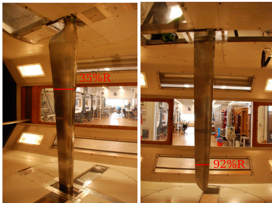
Fig. 4. Two experimental setups for the non-rotating MEXICO blade measurement in the low speed low turbulence wind tunnel of Delft University of Technology.
