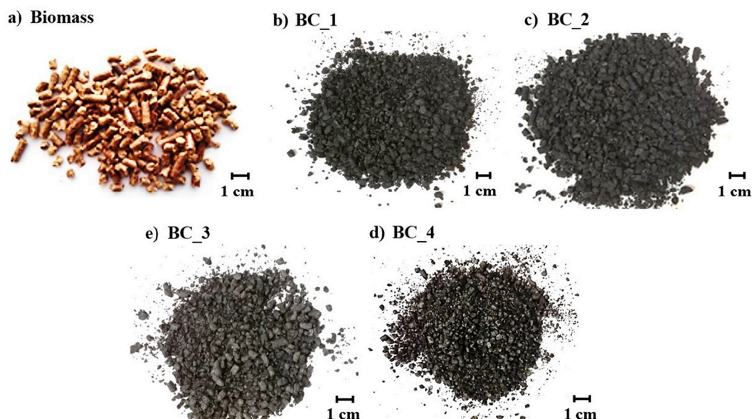
Fig. 1. Biomass and biochars studied in this work. a) Biomass, b) BC_1 ( T = 850 °C, \lambda = 0.25 , SB = 0), c) BC_2 ( T = 850 °C, \lambda = 0.30 , SB = 0), d) BC_3 ( T = 836 °C, \lambda = 0.20 , SB = 0.80) and e) BC_4 ( T = 840 °C, \lambda = 0.20 , SB = 1.20).
