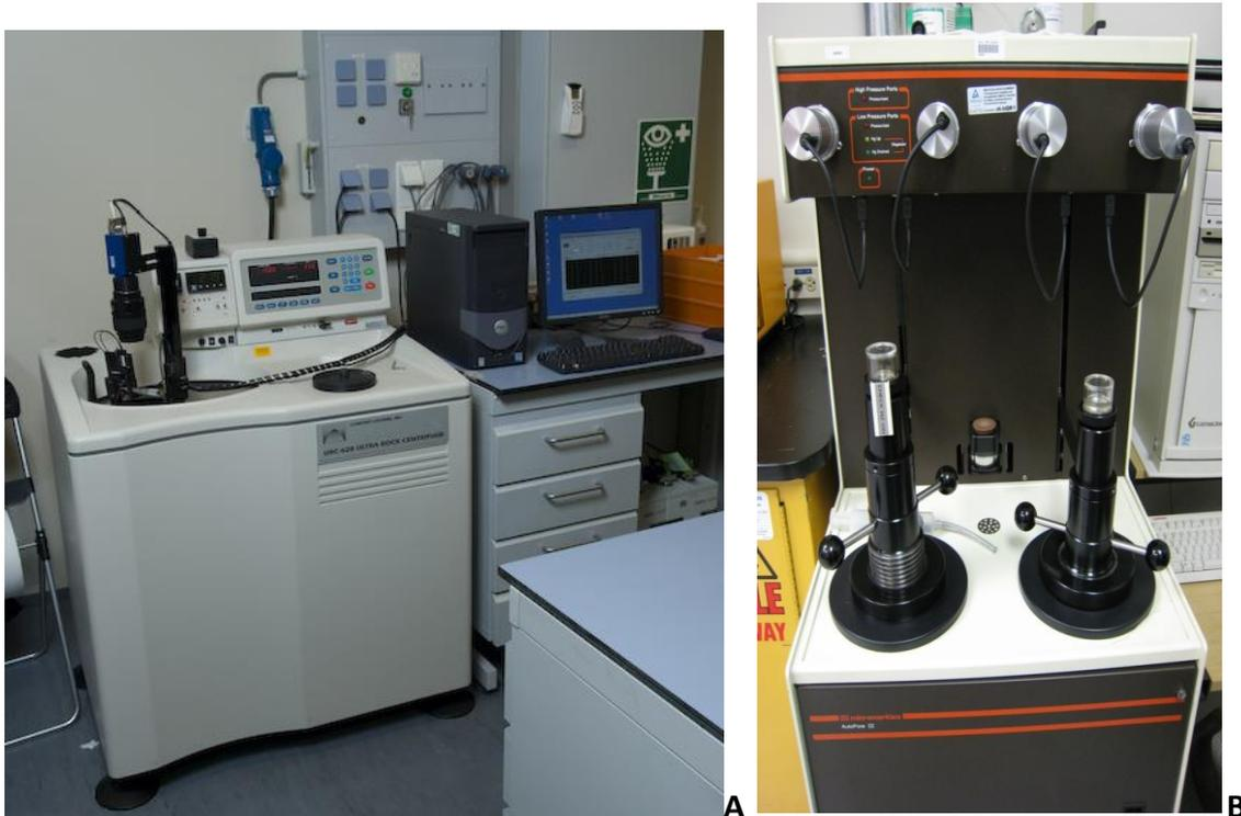
Figure 2.7: A: Centrifuge experiment, B: Micromeritics autopore IV
