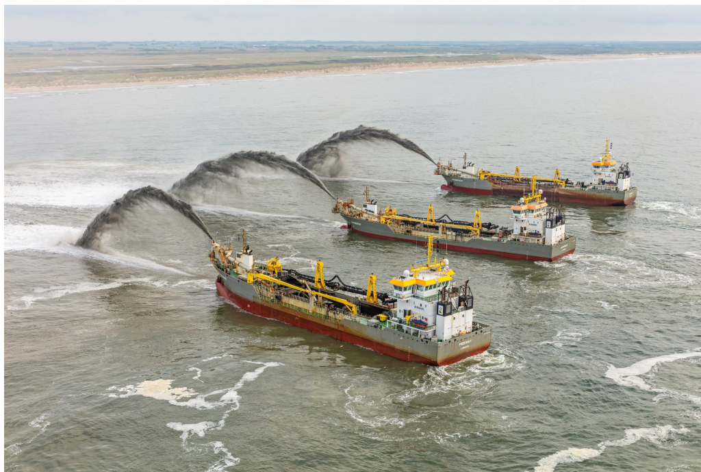
Figure 1.2: Coastal replenishment with three THSDs rainbowing [29]
