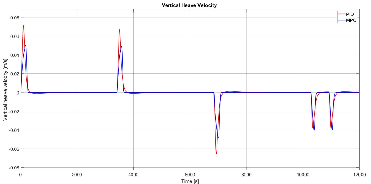
Figure 6.30: Comparison of the heave velocity for PID and MPC
