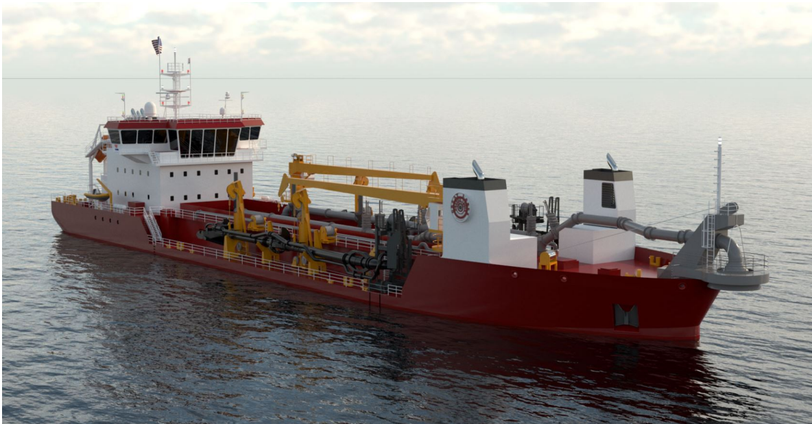
Figure 6.35: Conventional dredger used as reference ship
