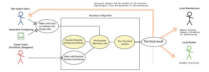
the objectives of the thesis are to design an interactive tool for normal users to customize their modular architecture from the input voxel array. Second, offering a structural validity check of the frame generated. Third, offering architectural tiles that incorporate mass customization enables expert users to develop the tileset using the framework.
