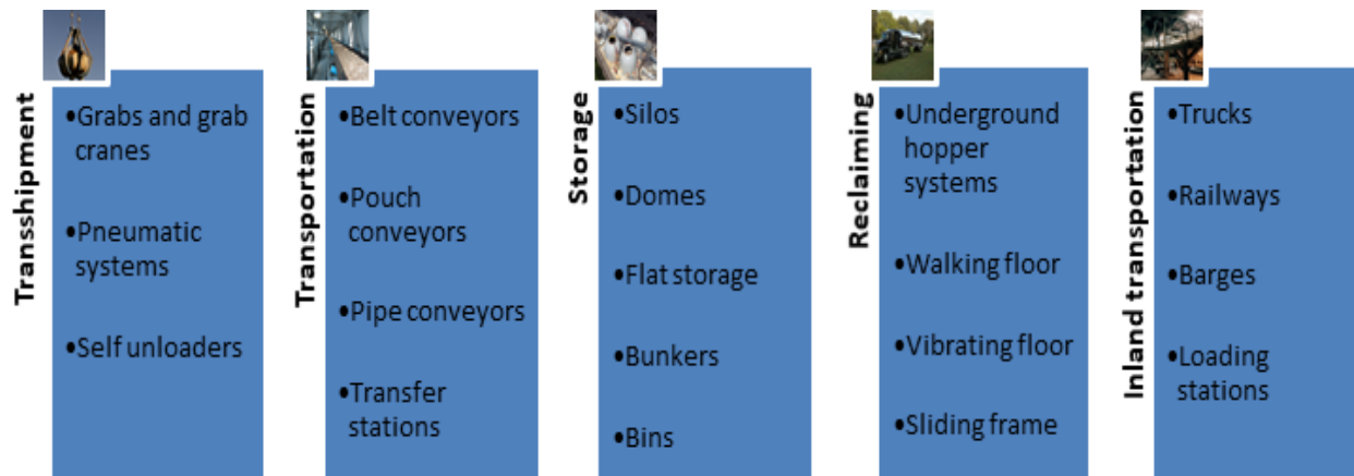
Figure 4.2: Example of solid biomass handling equipment [3]
