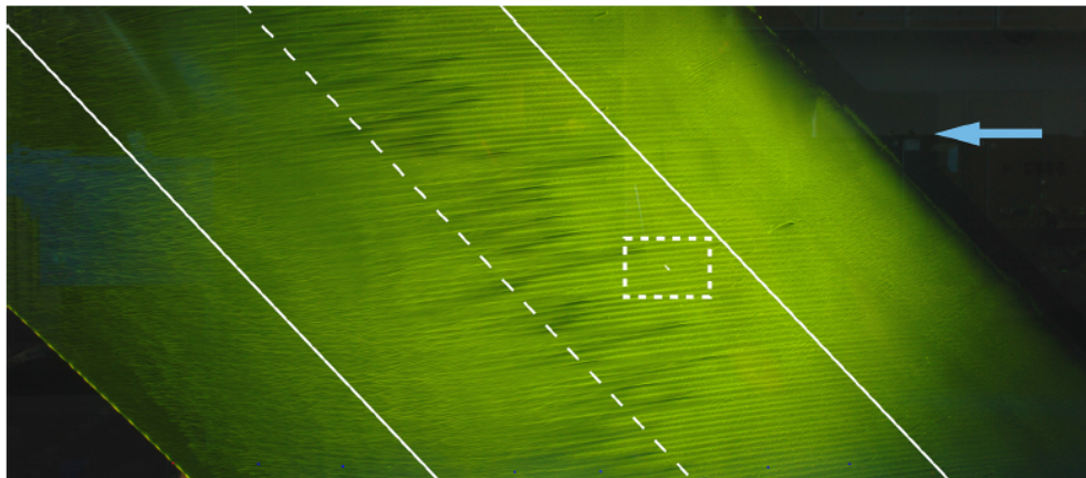
Figure 3.4: Sawtooth transition front observed in fluorescent oil flow visualization. Flow comes from the right (indicated by blue arrow). Re = 2.12 \times 10^6 , \alpha = 3^\circ . White dashed line indicates the wing mid section x/c = 0.50 . Left solid white line indicates x/c = 0.75 and right solid white line indicates x/c = 0.25 . (reproduced from [33])
