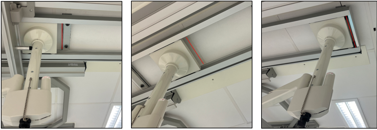
Figure 25: Show the reference positions of the lead shield during the second part of the visualization measurements. Left: position 1 closes to the phantom. Middle: position 2 the middle position of the lead shield. Right: Position 3 the furthest away from the phantom.
