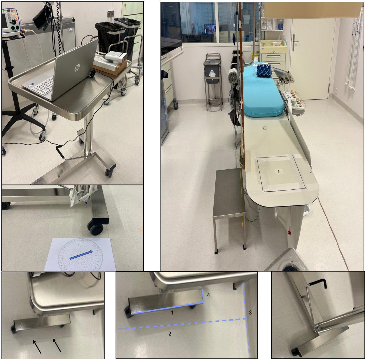
Figure 22: Showing the setup in the Cath lab. A: The placement of the elevated Azure Kinect DK with the laptop that controls it. B: The surgeon's table where the phantom and the center are marked exactly in the middle. C: Shows how the orientation of the setup table for the Azure Kinect and the laptop is validated. D: Showing a line in the Cath lab as a reference position of the table for the Azure Kinect. E: The lines in the Cath lab are numbered for the positioning of the table for the Azure Kinect. Line 1 is positioned over line 2, so the lines are parallel. Line 4 is positioned parallel to line 3 at a certain distance. F: The bar handle is shown to adjust the orientation of the tabletop.
