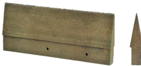
Figure 1.6: Metal foam trailing-edge insert for airfoil noise reduction [14].
