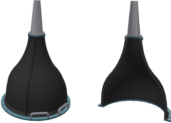
Figure B.3: Full constructive design of the nozzle with attachment to the tunnel circuit and internal frames in the contraction section.
