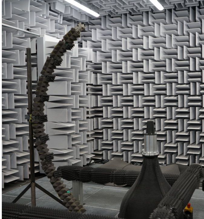
Figure B.4: Jet nozzle mounted in the anechoic chamber with microphone arc-array.
