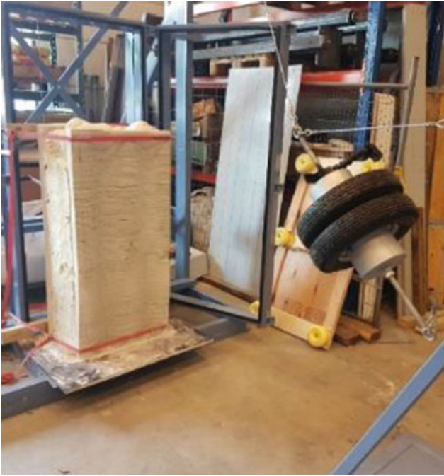
Fig. 6.19 Impact test (Bos et al. 2019)
