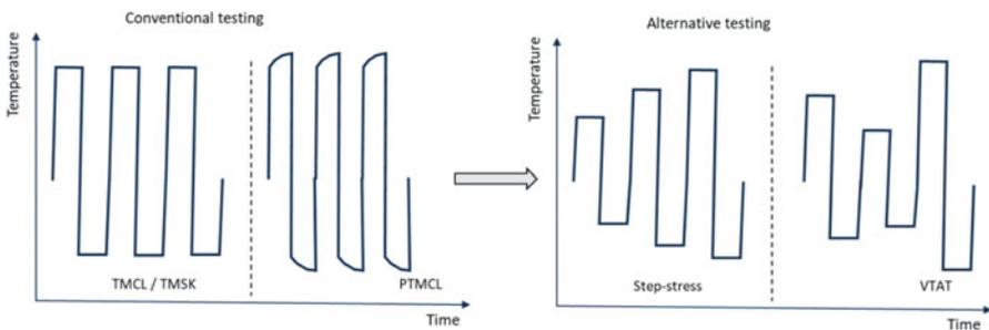
Fig. 16.4 Conventional temperature cycling (TMCL) or temperature shock (TMSK) and power temperature cycling (left) versus alternative temperature testing: step-stress or variable temperature accelerated testing
