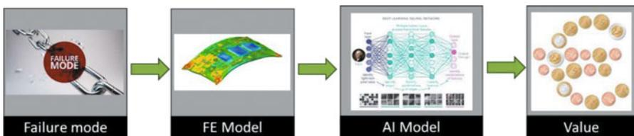
**Fig. 16.5** Starting from a failure mode, a finite element analysis will be set up, and results are fed into the AI model which on its turn creates value as it enables lifetime prediction of each possible design
