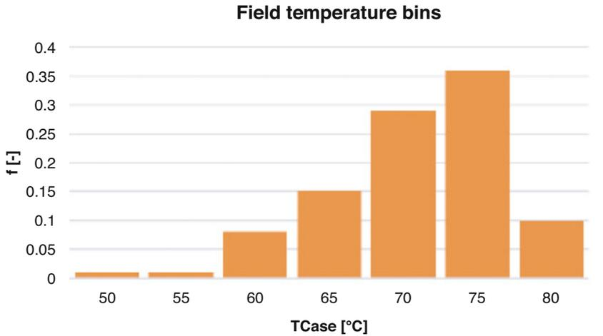
Fig. 16.3 Typical temperature occurrences (frequencies) in electronics
