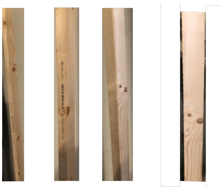
Figure 8.4: A-symmetric fibres and knots causing anisotropy in the timber columns.
