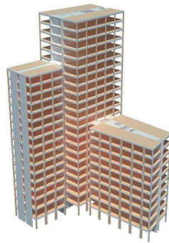
Figure B.11: Structural system HoHo Wien [9].
