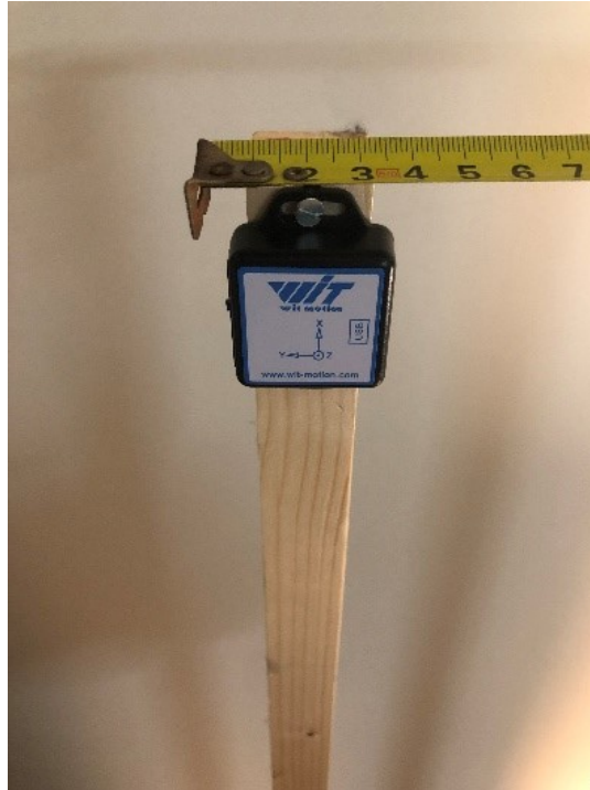
Figure 7.6: The accelerometer used in the experiments.
