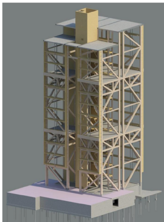
Figure B.5: Glulam truss system Treet [33].
