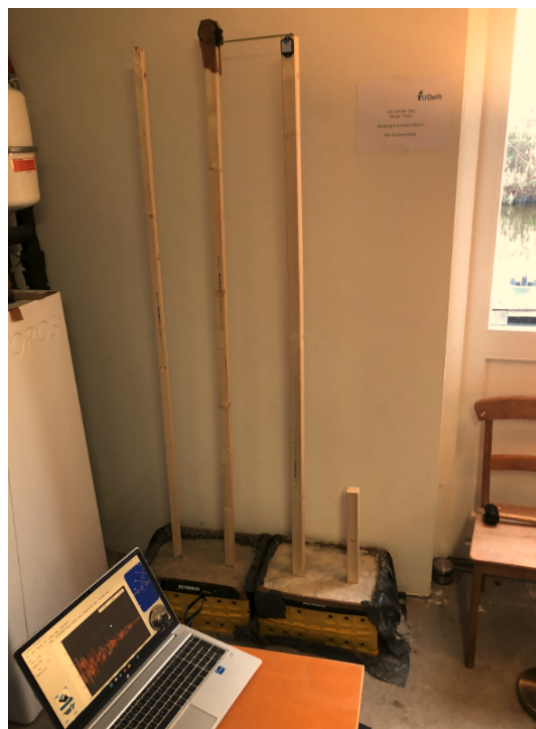
Figure 7.4: The physical models: four clamped columns. Note that the adopted set-up numbering 1 - 4 is in the picture from right to left; the column on the right is the stiffest (setup 1), ending with the most flexible (setup 4) on the left.
