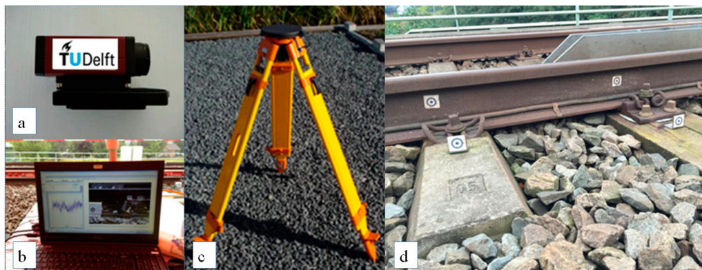
Figure 4. A DIC-based device: (a) a high-speed camera; (b) processing system; (c) a tripod; (d) targets.
