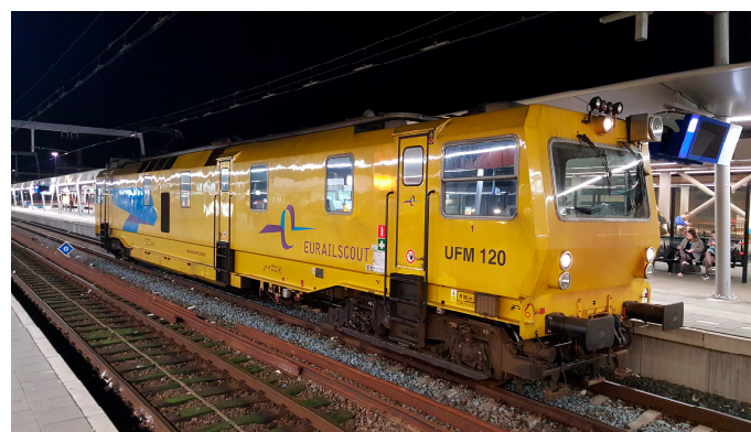
Figure 3. EURAILSCOUT UFM120 measuring coach [48].
