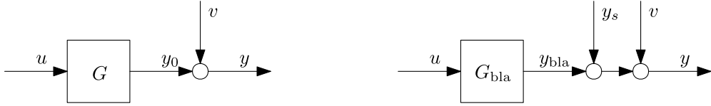
Fig. 4. The BLA represents a nonlinear system G using a LTI contribution G_{\text{bla}} , a stochastic nonlinear contribution y_s , and a noise source v .
