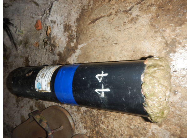
Figure B.8: A wave logger with barnacles. Photograph by Celine van Bijsterveldt, March 2018.
