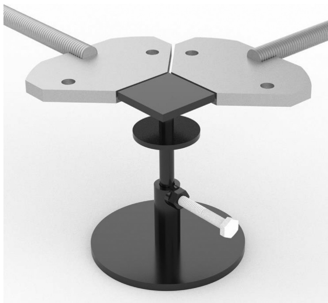
Fig. 13. The adjustable temporary support for the samples to be used during clamping.
