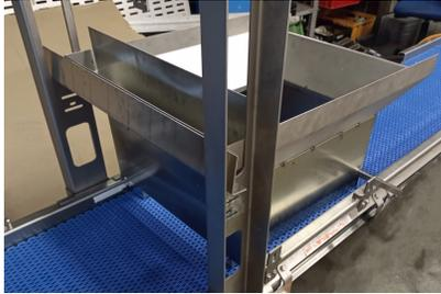
Fig. 12: The bulk experiment test setup, the height of the opening near the conveyor is adjustable.
