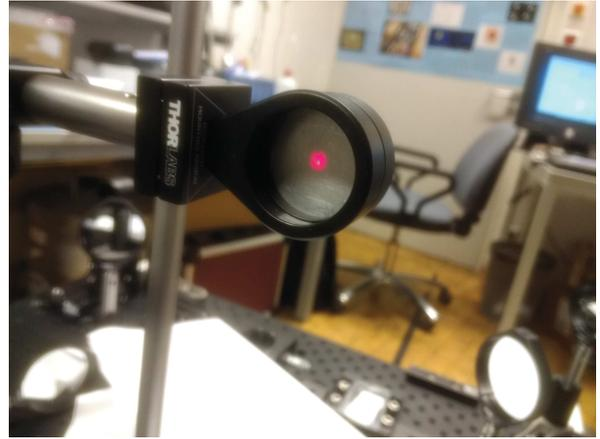
Figure 4.15: To ensure that the optical beam reflected by the dichroic window was aligned with the optical axis, it had also to pass through the centre of the  $f = 750\text{ mm}$  Ge lens, already aligned with the optical axis, which for convenience was replaced with a  $\sim 1\text{ mm}$  circular aperture.
