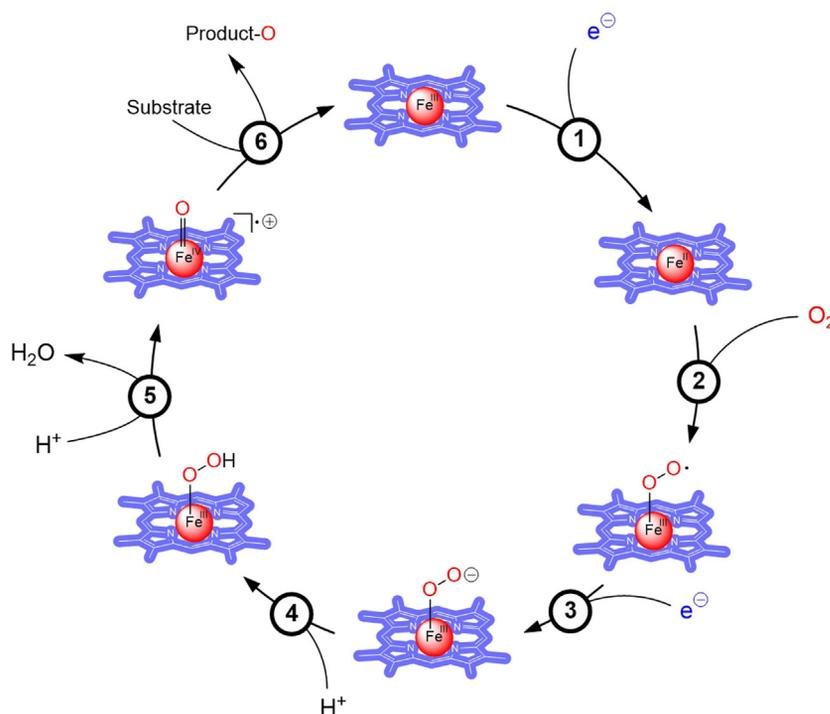
**Figure 23. Simplified mechanism of P450-catalyzed oxyfunctionalization reactions**
