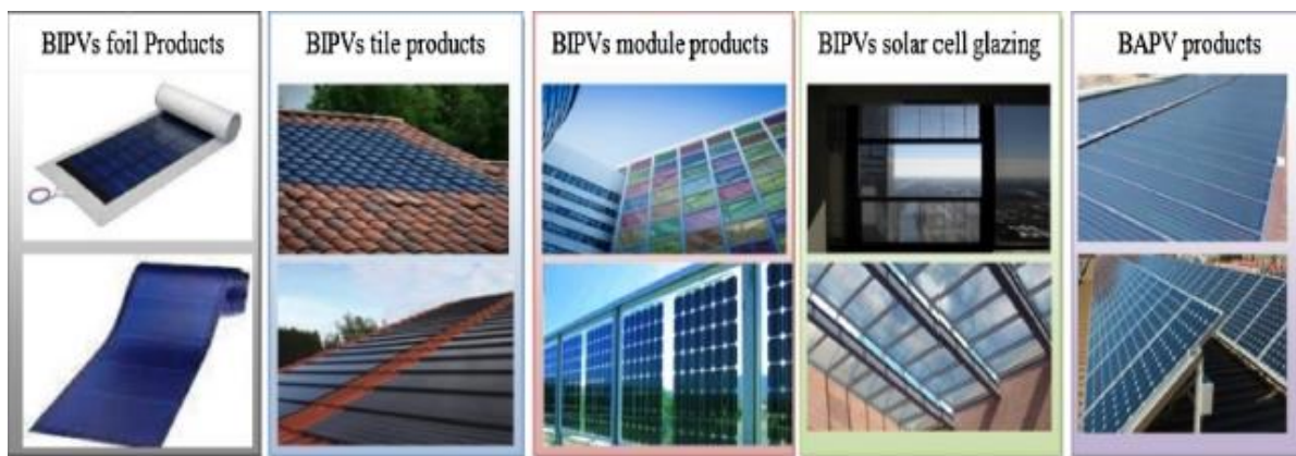
Figure 2.9 Classification of BIPVs Product [17]
