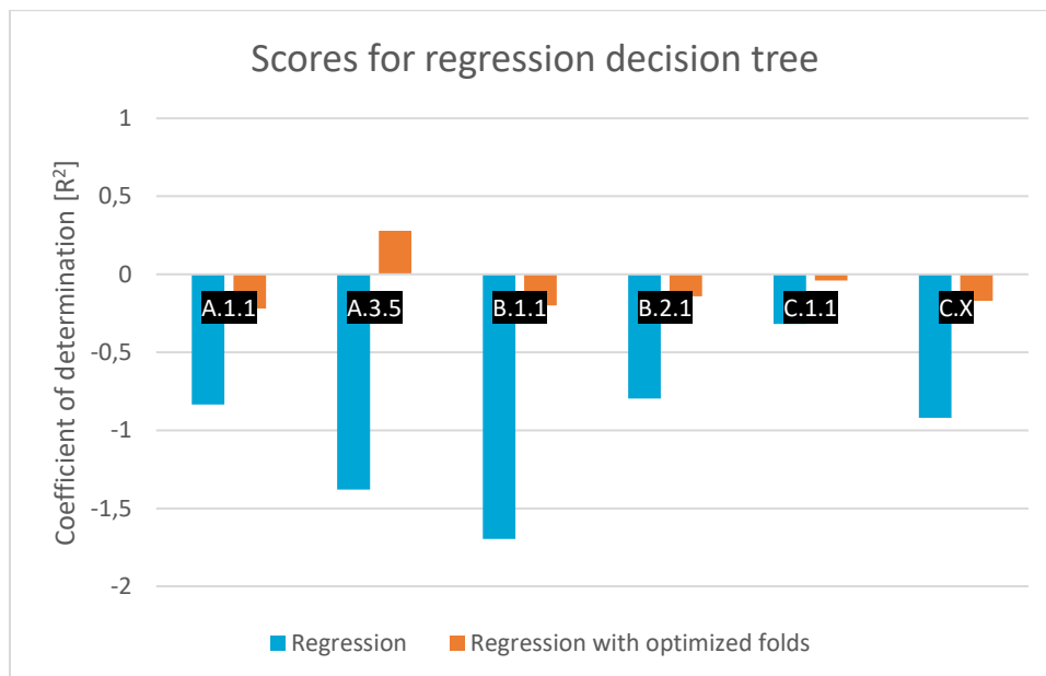
Figure 35 Consequences of optimizing the number of folds in the GKF cross-validation on the coefficient of determination.
