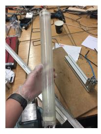
(b): The shrink sleeve is pulled over the im- (c): The STEM after curing and removing pregnated glass fibre sleeve. from the mould. The ends remain to be cut.
