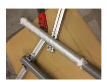
(a): The glass fibre sleeve is fixed onto the PVC mould
