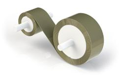
(b): An example of a constant torque spring. By winding the free end of the spring onto a secondary drum, the constant force spring is transformed into a constant torque spring. Image courtesy of Vulcan [?].
