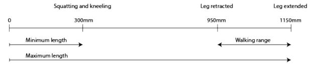
Figure 2.7: A visualisation of the range of lengths that the device should facilitate. The minimum length occurs while kneeling while the maximum length occurs when the leg just touches the ground during walking.
