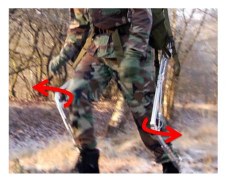
Figure 1.2: The legs of the Exobuddy tend to rotate outward during operation, increasing the risk of collision with obstacles.
