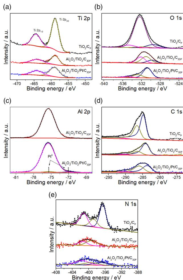
**Figure 4.** XPS spectra of a) Ti 2p, b) O 1s, c) Al 2p, d) C 1s, and e) N 1s of the pyrolyzed samples  $\text{TiO}_2/\text{C}_\text{P}$ ,  $\text{Al}_2\text{O}_3/\text{TiO}_2/\text{C}_{3\text{DP}}$ , and  $\text{Al}_2\text{O}_3/\text{TiO}_2/\text{Pt}/\text{C}_{3\text{DP}}$ .
