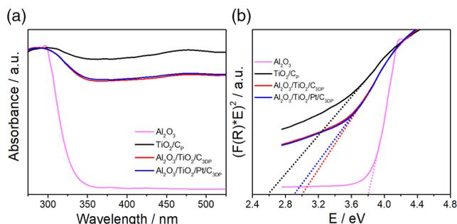
**Figure 5.** a) UV-vis absorption spectra and b) Tauc plots of pristine  $\gamma-Al_2O_3$ , Ti-MOF-derived  $TiO_2/C_p$ , and 3D-printed boehmite/Ti-MOF-derived  $Al_2O_3/TiO_2/C_{3DP}$  and  $Al_2O_3/TiO_2/Pt/C_{3DP}$ .
