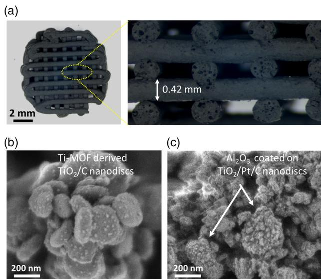
**Figure 1.** a) Optical image of pyrolyzed 3D-printed  $\text{Al}_2\text{O}_3/\text{TiO}_2/\text{Pt}/\text{C}_{3\text{DP}}$  monolith. Right-hand enlarged image is the cross-sectional view of the monolith. SEM images of b) Ti-MOF-derived  $\text{TiO}_2/\text{C}$  and c) Pt-deposited boehmite/Ti-MOF-derived  $\text{Al}_2\text{O}_3/\text{TiO}_2/\text{Pt}/\text{C}_{3\text{DP}}$ .
