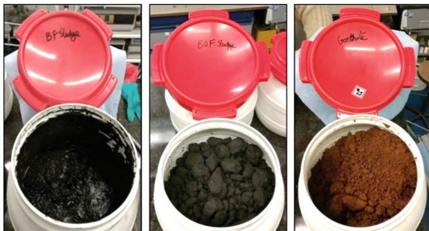
Fig. 1 As-received material in the wet form, from left-to-right BF dust, BOF dust, and goethite
