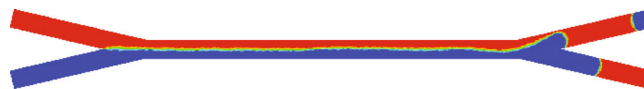
FIGURE 12 Parallel flow for water-toluene mixture simulated using VOF and VOF-LS. The red fluid is water and the blue fluid is toluene. [Colour figure can be viewed at wileyonlinelibrary.com]
