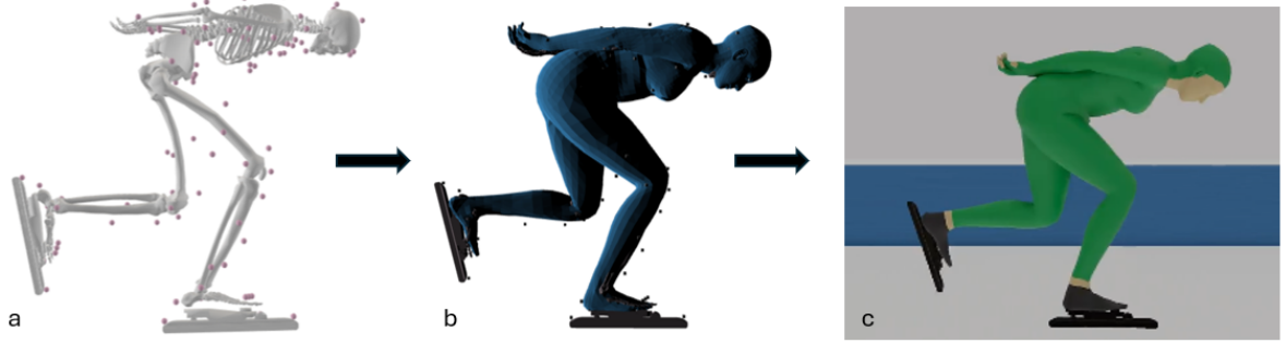
Figure 3: Overview of the pipeline: a. OpenSim skeletal model b. Fitted SMPLX mesh c. Rendered image of same pose
