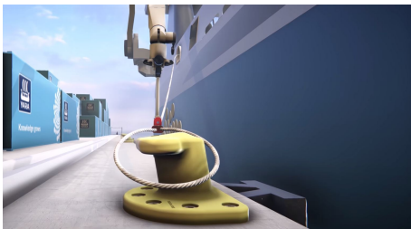
Figure 4.1.1: McGregor mooring system used in the Yara Birkeland [65]
