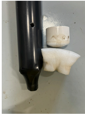
(b) Step 3: Plugging the well
