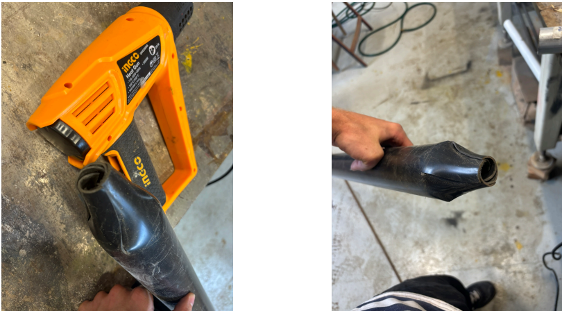
Figure C.2: Well tip shaped with heatgun
