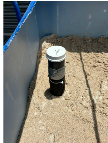
(c) Step 4: Top of the well, sealed
