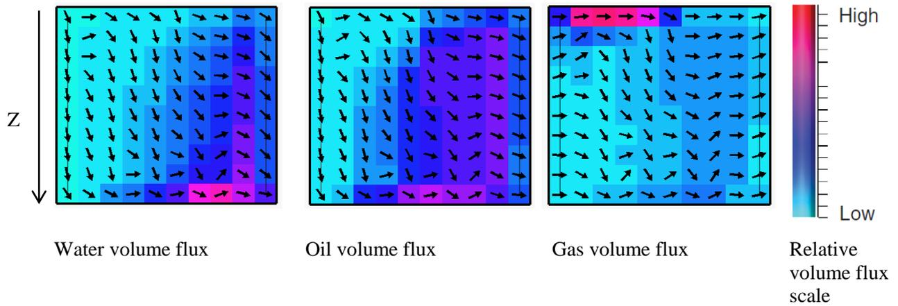
**Figure 5** SAG process in a 2D reservoir, with dimensions 1m x 100m x 30m, and modeled with 1 X 10 X 10 gridblocks. These figures show the net volume fluxes of the phases between the gridblocks at reservoir conditions at the end of the simulation. Switching time = 1.63 PV, gas injection period = 100 days, equal to 0.49 PV
