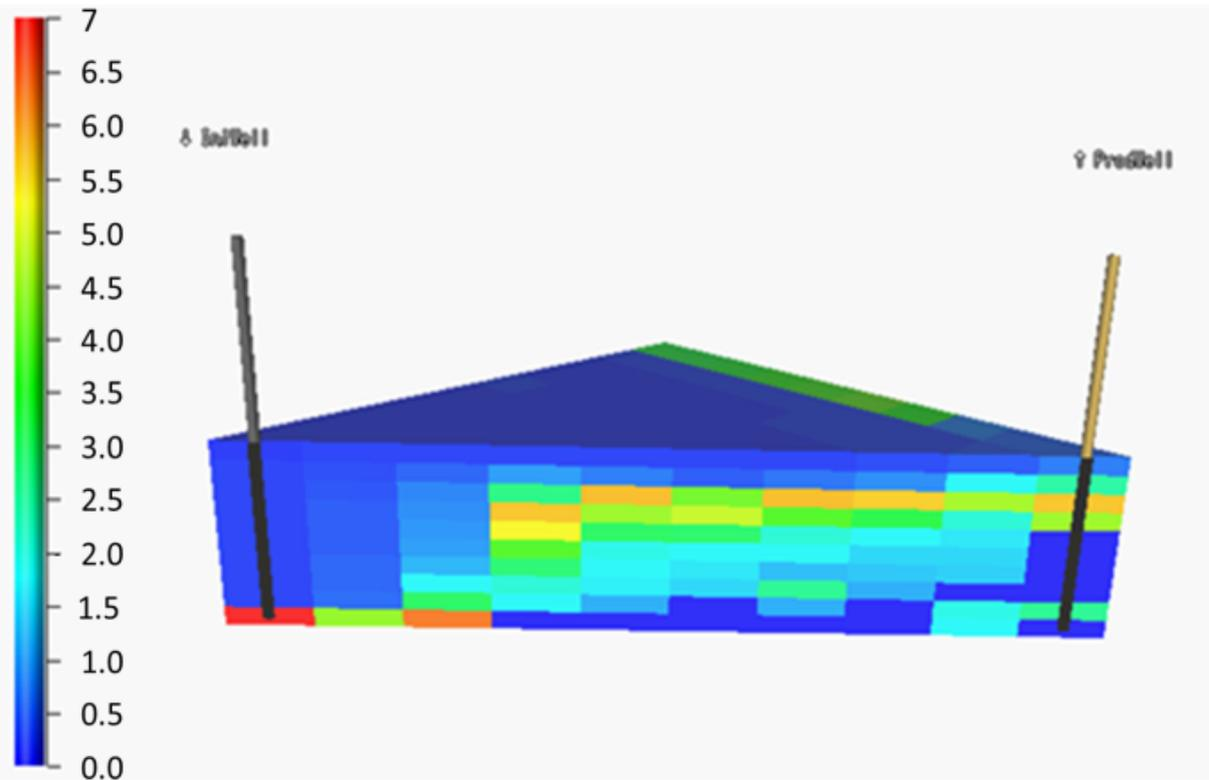
**Figure 2** Gas viscosity (cP) at the end of the simulation, for switching time = 0.37 PV, and gas injection time = 250 days, equivalent to 0.64 PV. In this figure and those to follow, the initial oil saturation is 0.3
