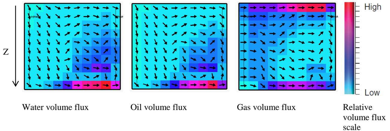
**Figure 6** SAG process in a 2D reservoir, with dimensions 10m x 100m x 30m, and modeled with 1 X 10 X 10 gridblocks. These figures show the net volume fluxes of the phases between the gridblocks at reservoir conditions at the end of the simulation. Switching time = 1.63 PV, gas injection period = 250 days, equal to 2.21 PV
