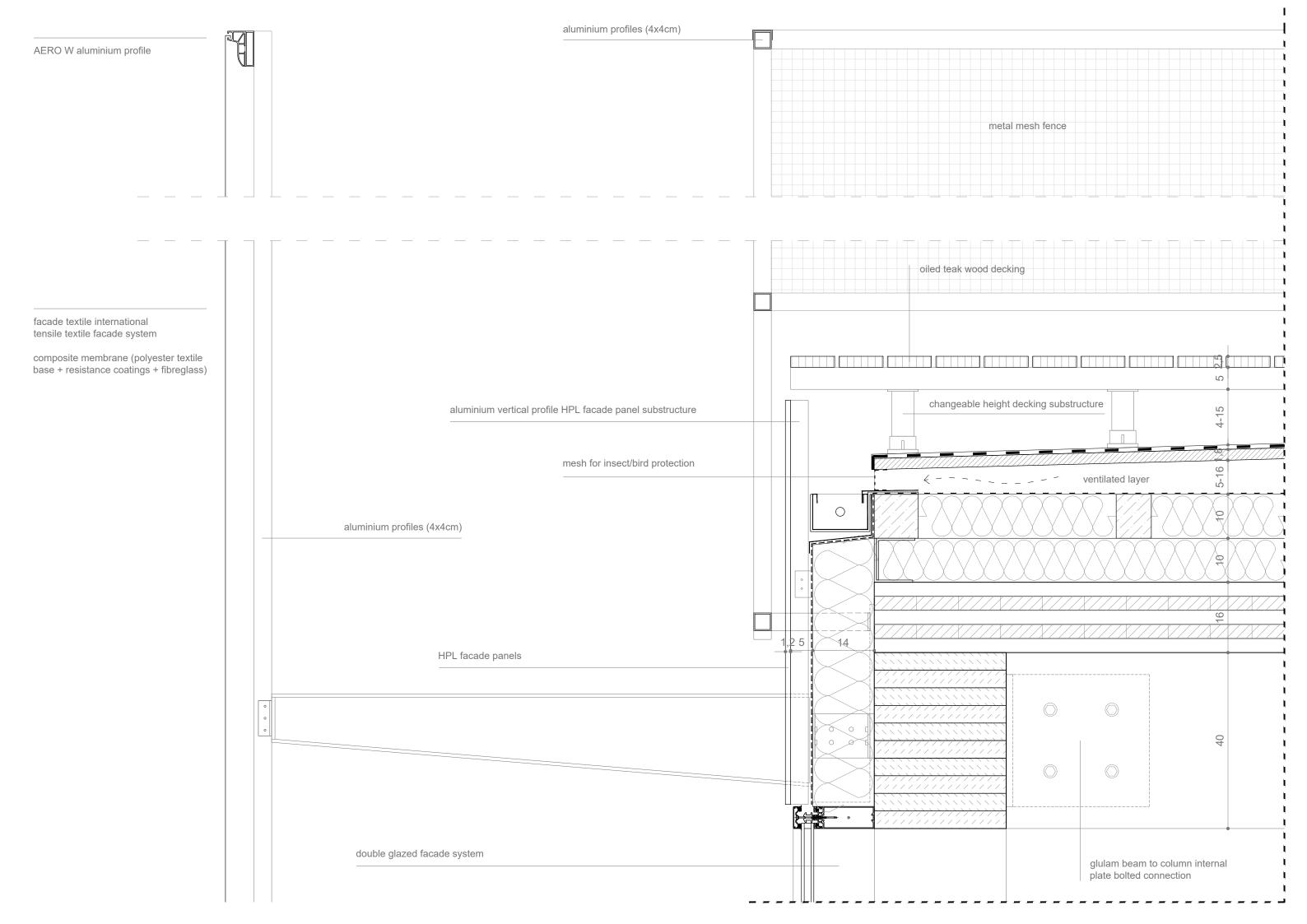
floor heating / cooling system facade textile international double glazed facade system tensile textile facade system composite membrane (polyester textile base + resistance coatings + fibreglass) ceramic tiles in glue EPS-T sound insulation aluminium profiles (4x4cm) expanded metal mesh 14 14 recycled textile insulation AERO W aluminium profile HPL panels aluminium hanging substructure
