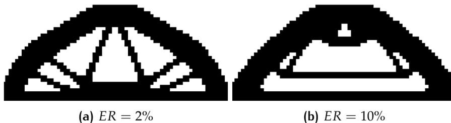
Figure 2.12: Comparison between results for different ER
