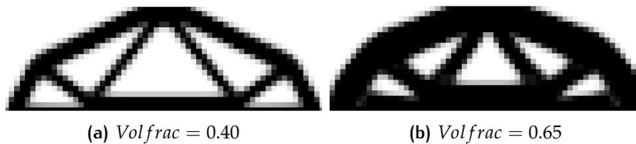
Figure 2.9: Comparison between results for different values of  $Volfrac$
