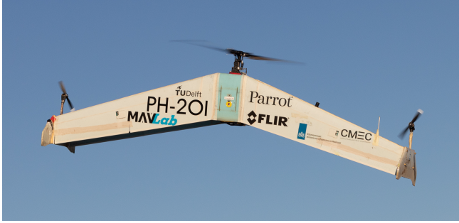
Figure 2: DelftaCopter in hover. In forward flight, the entire fuselage pitches down 90^\circ and the rotor provides the thrust as shown in Figure 1.
