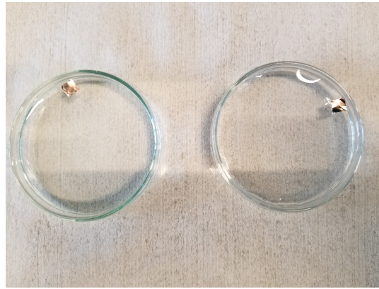
Figure 4.1: Image of two pieces of graphene along with the copper foil floating on the surface of the APS solution in separate petri dishes.
