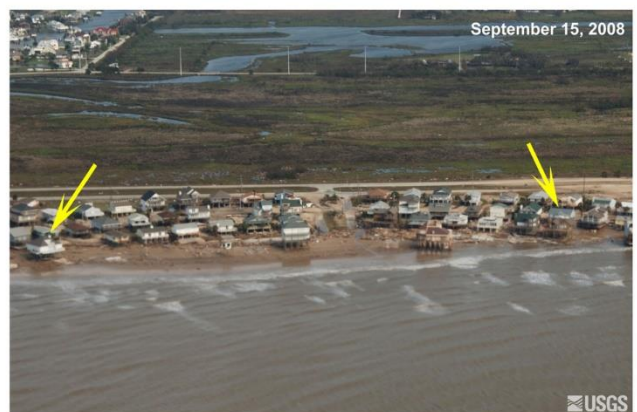
FIGURE 5.3.6. PRE- AND POST-IKE AERIAL PHOTOGRAPHS OF SECTIONS OF THE WEST END AREA. THE LEFT PANEL SHOWS THE AREA THAT CORRESPONDS WITH TRANSECT A. INDICATED WITH THE YELLOW ARROW IS THE DELLANERA RV PARK. IT IS CLEAR THAT AREA IS HEAVY REINFORCED AND DID NOT ERODE DURING THE STORM. THE RIGHT PANEL SHOWS THE AREA THAT CORRESPONDS WITH TRANSECT B. THE SHORELINE HAS RETREATED DUE TO HEAVY EROSION WHEN IKE MADE LANDFALL. HOWEVER PRIVATE PROPERTIES PREVENTED FROM FURTHER EROSION (USGS, 2009).
