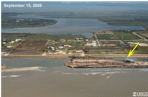
FIGURE 5.3.6. PRE- AND POST-IKE AERIAL PHOTOGRAPHS OF SECTIONS OF THE WEST END AREA. THE LEFT PANEL SHOWS THE AREA THAT CORRESPONDS WITH TRANSECT A. INDICATED WITH THE YELLOW ARROW IS THE DELLANERA RV PARK. IT IS CLEAR THAT AREA IS HEAVY REINFORCED AND DID NOT ERODE DURING THE STORM. THE RIGHT PANEL SHOWS THE AREA THAT CORRESPONDS WITH TRANSECT B. THE SHORELINE HAS RETREATED DUE TO HEAVY EROSION WHEN IKE MADE LANDFALL. HOWEVER PRIVATE PROPERTIES PREVENTED FROM FURTHER EROSION (USGS, 2009).
