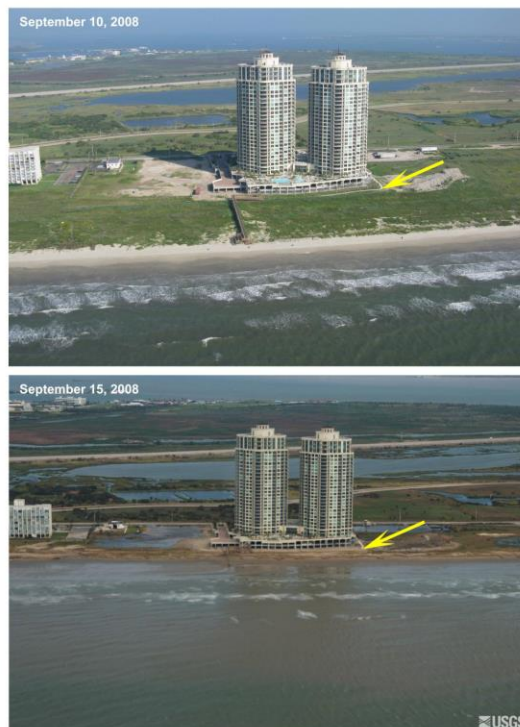
FIGURE 5.3.4. PRE- AND POST-IKE AERIAL PHOTOGRAPHS OF SECTIONS OF THE EAST BEACH AREA. THE PHOTO SHOWS THE PALISADE PALMS AND THE COASTLINE REGRESSION AFTER IKE. THIS REGION LIES BETWEEN TRANSECT B & C. (USGS, 2009).
