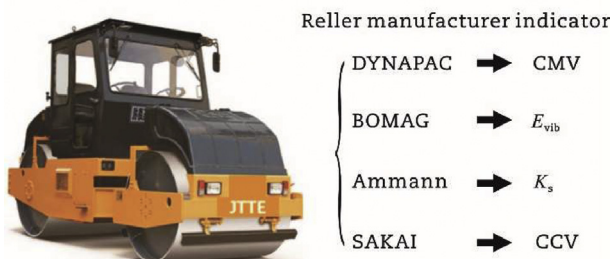
Fig. 88 – Types of compaction quality control index.
