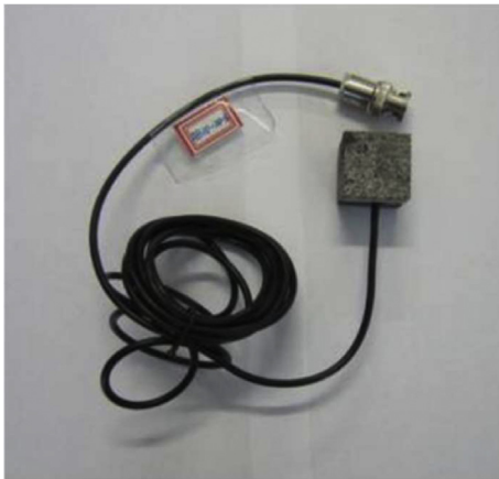
Fig. 62 – Intelligent sense aggregate (Jiang, 2013).
