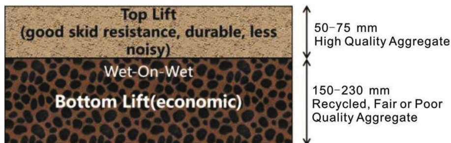
Fig. 24 – Structure diagram of 2LCP.
