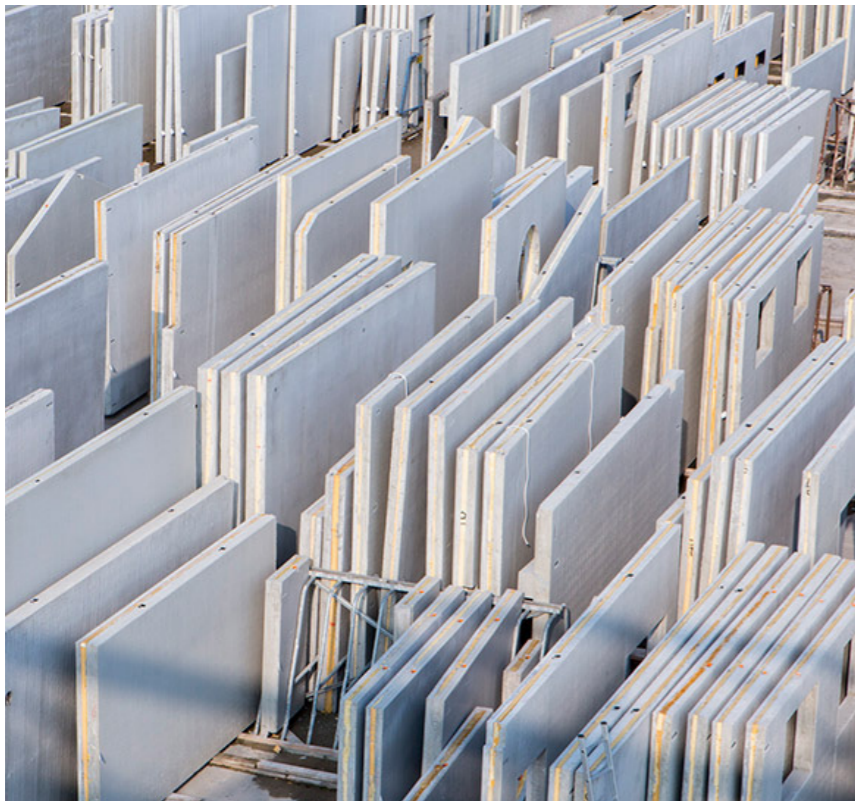
demountable prefab concrete elements for cores
