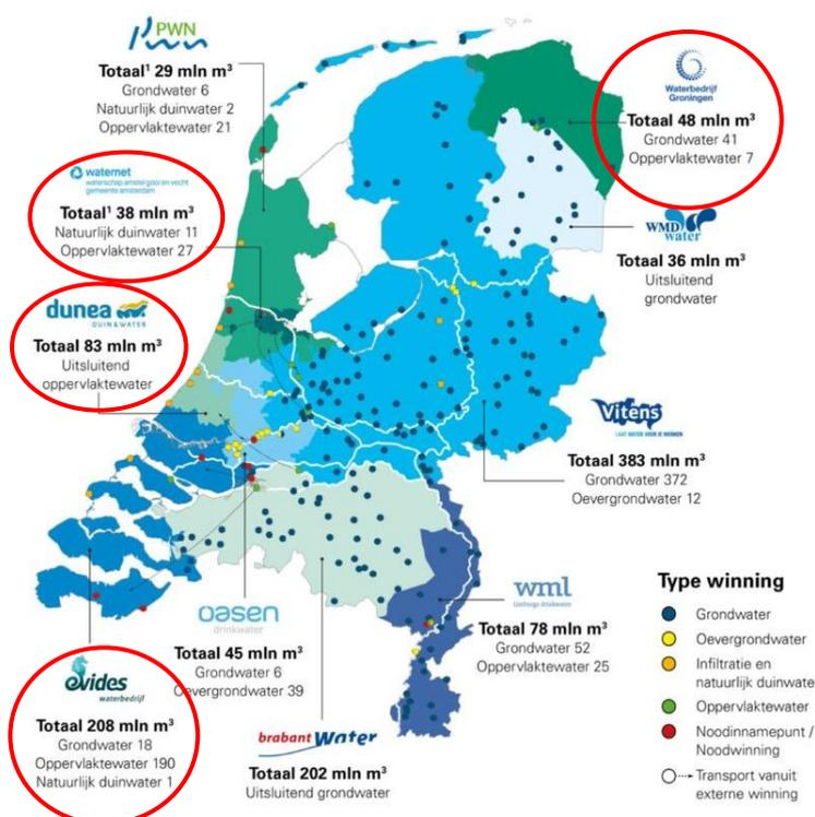
**Figure 3:** Map of Dutch drinking water companies with their distribution areas, sources, intake points and extracted water quantities (2018) [1]. Groundwater = groundwater, oevergrondwater = riverbank filtrate, infiltratie en natuurlijk duinwater = infiltrated and natural dune water, oppervlaktewater = surface water, noodinnamepunt = emergency extraction point, transport vanuit externe winning = transport from external extraction. Encircled the companies that provided data for this research.
