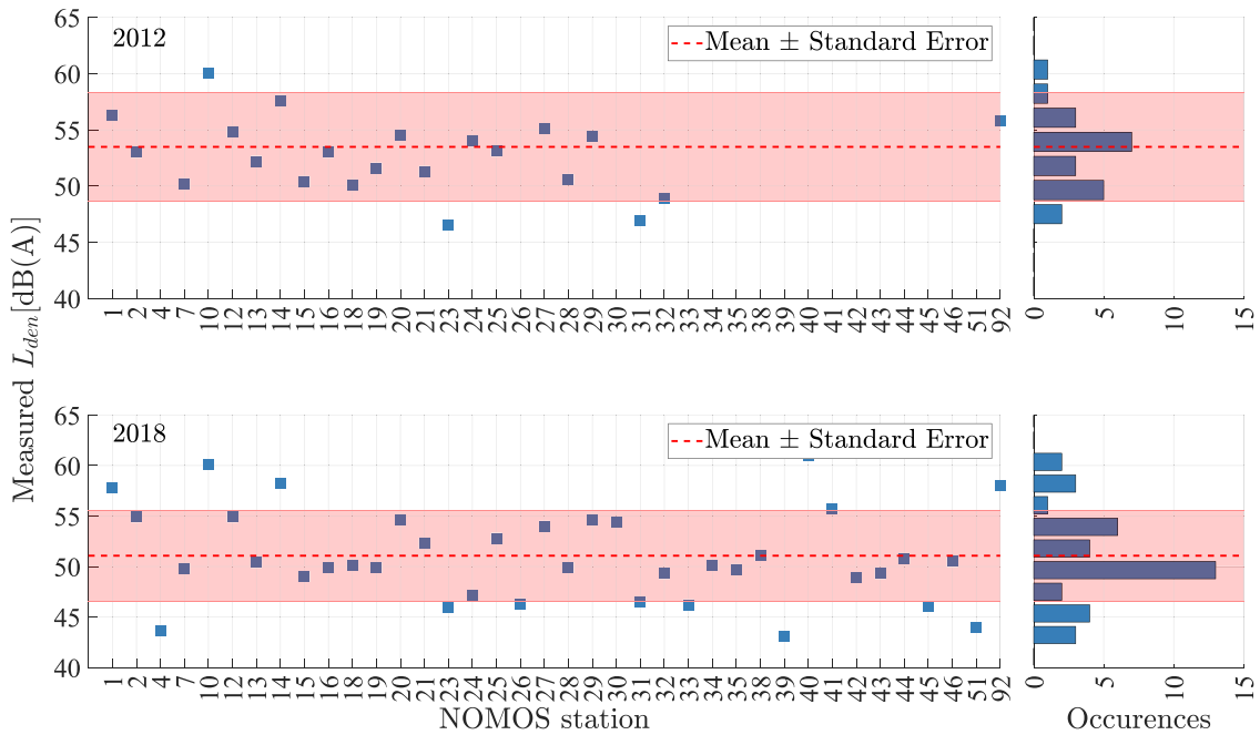
Fig. 5. Distribution of measured L_{den} data per NOMOS station for the years 2012 (top) and 2018 (bottom). The plots contain a scatter plot of all NOMOS stations (blue squares), and a distribution of these measured L_{den} with the mean as a dashed red line and the spread in red background.
