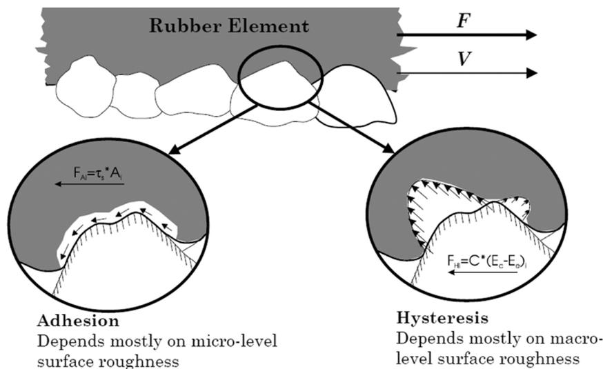
Fig. 1. Schematics of adhesion and hysteresis [7].
