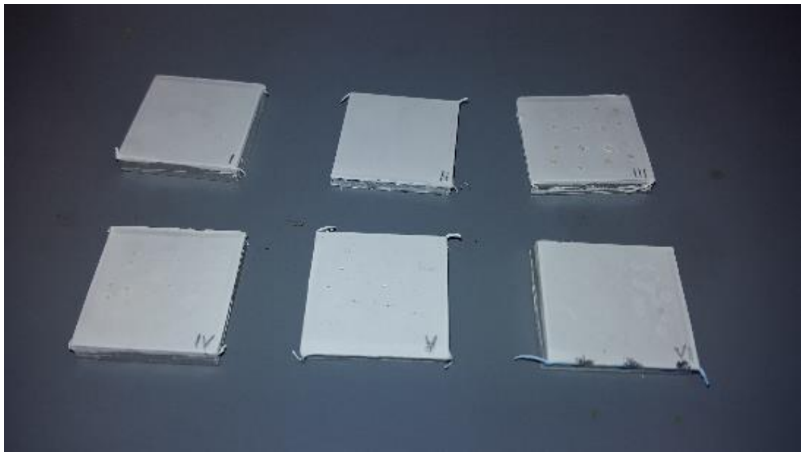
Alginate droplets deposited on spincoated PVDF thin film on glass before it had fully dried, creating streaks around the alginate droplets. A crater shaped microrelief could be found under the cured alginate drop after detachment from the fully dried PVDF film.
