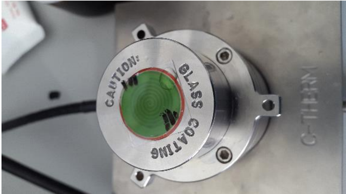
Top-down placement of a glass sample, spincoated with a PVDF thin film.
