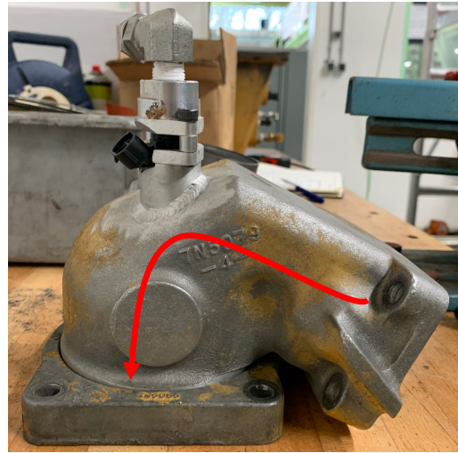
Figure 2: Airflow through inlet air receiver [9]
