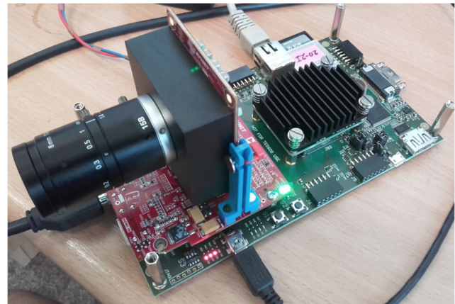
Figure 8 Evaluation setup consisting of a Trenz carrier board with Xilinx Z0720 SoM and Python 1300 camera on a HDMI I/O board.
