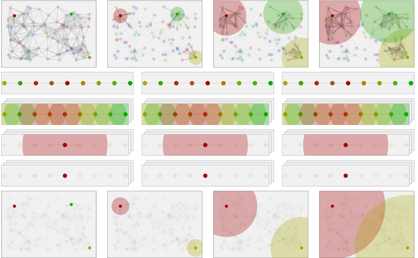
Fig. 4. Multinode aggregation graph neural networks. Start by selecting a subset \mathcal{P}_1 \subset \mathcal{V} of P_1 nodes of the graph (row 1, diagram 1). Then, proceed to perform Q_1 local exchanges with neighbors (row 1, diagrams 2, 3, and 4) in order to build P_1 regular time-structure signals, one at each node (row 2), see (22). We note that in row 1, the color disks illustrate the reach of the Q_1 local exchanges of each of the selected nodes \mathcal{P}_1 . Once the regular structured signals have been constructed on each of the P_1 nodes, proceed with a regular CNN, applying regular convolution (row 3), and regular pooling (row 4), until F_{L_1} features are obtained at each node (row 5), see (2)–(5), (23). Now, we view each feature as a graph signal being supported on the selected nodes, see (24), zero-padded to fit the graph (row 6, diagram 1), see (25). We then select a smaller subset \mathcal{P}_2 \subset \mathcal{P}_1 of P_2 \leq P_1 nodes (row 2, diagram 2) and carry out Q_2 local exchanges with the neighbors, (row 2, diagrams 2, 3 and 4), illustrated with color disks in the last row. These neighbor exchanges create new regular structured signals at each of the \mathcal{P}_2 nodes, see cf. (26). Then, we continue by computing F_{L_2} regional features at each node by means of regular CNNs and so on.
