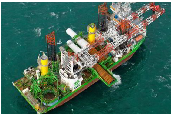
(a) Typical lay out of an installation ship. One monopile is resting in the up-end tool. The yellow transition pieces are standing on the deck.
