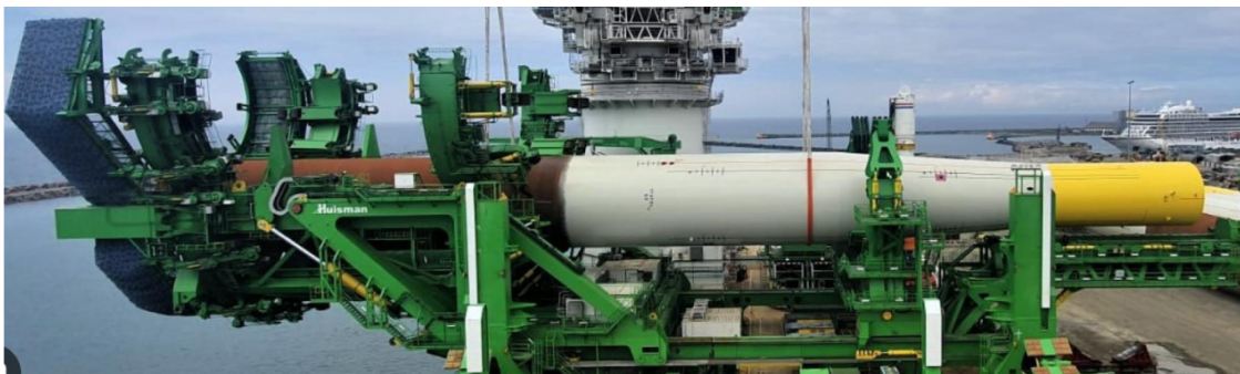
Figure 6.4: A monopile lying down in the upending tool. The support pads need to avoid contact with the appendages.
