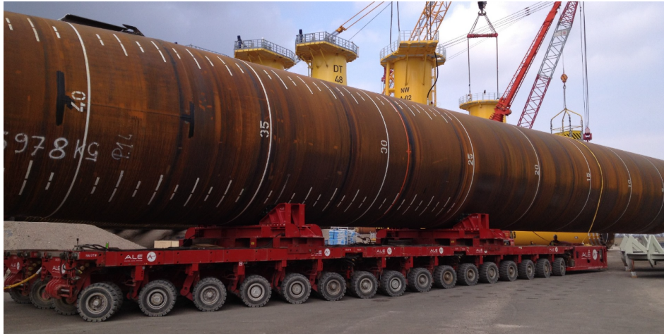
Figure 6.3: A monopile on a SPMT during transshipment. The circular support stands are clearly visible. It also can be seen that it stick out more than 20 m.
