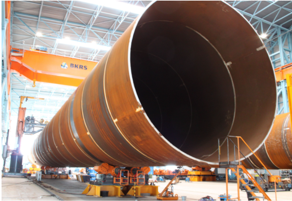
Figure 6.2: Monopile on rollers in the production hall.
