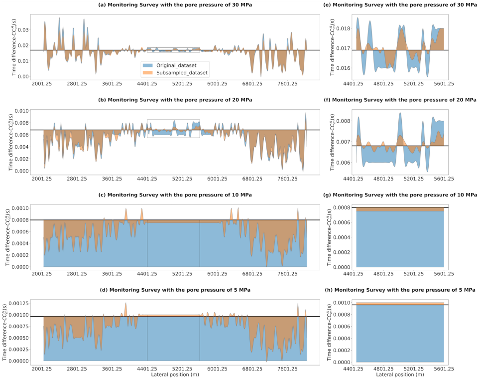
Figure 3.6: The retrieved time differences in the reservoir using ghost reflections for the monitoring surveys with pore pressure of (a) 30 MPa, (b) 20 MPa, (c) 10 MPa, and (d) 5 MPa for all virtual receivers. (e), (f), (g), and (h) Zoomed in results from inside the black rectangles in (a), (b), (c), and (d), respectively. The blue highlighted area shows the time difference using the original dataset, and the orange one shows the time difference using the intersampled dataset. The horizontal black lines show the calculated time differences.
