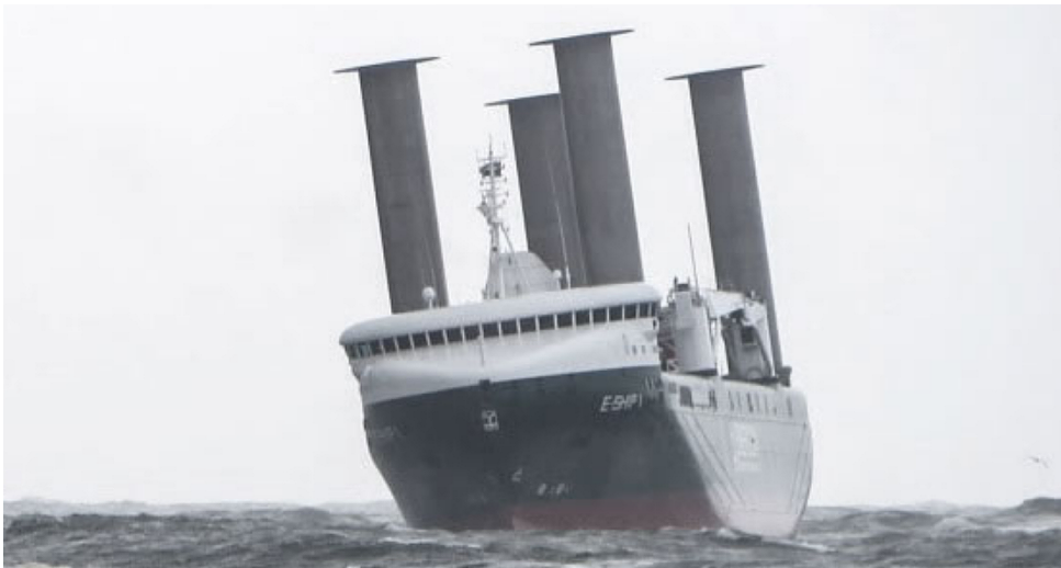
Figure 6.1.: E-Ship1, a 10500 DWT RoLo equipped with four 27 m Flettner rotors. In operation since 2010. (source: www.enercon.de ).
