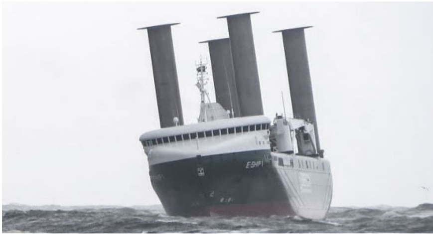
Figure 1.2.: E-Ship 1, equipped with four Flettner rotors, has been in commercial operation for nine years.
