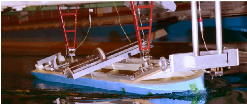
(a) Sailing yacht experimental setup for 2015 campaign.
