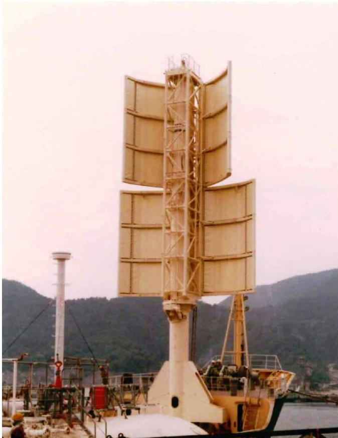
Figure 1.1.: JAMDA sail installed on coastal freighter in Japan (1980)
