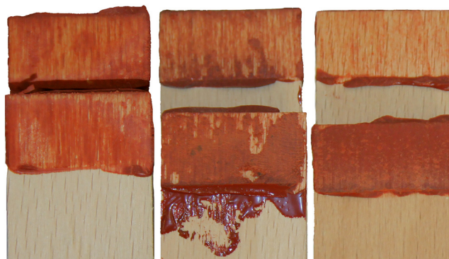
Fig 7. Example of failure modes through examination of the bonded surfaces after lap shear test completion. Left: cohesive (250 mg rosin/250 mg beeswax/50 mg ochre), the adhesive remains evenly bonded to both sides; middle: mixed-mode (400 mg rosin/100 mg beeswax/100 mg ochre), the adhesive favours one side, but remains bonded to both some areas; right: adhesive failure (400 mg rosin/100 mg beeswax/50 mg ochre), the adhesive remains bonded to one side only.
