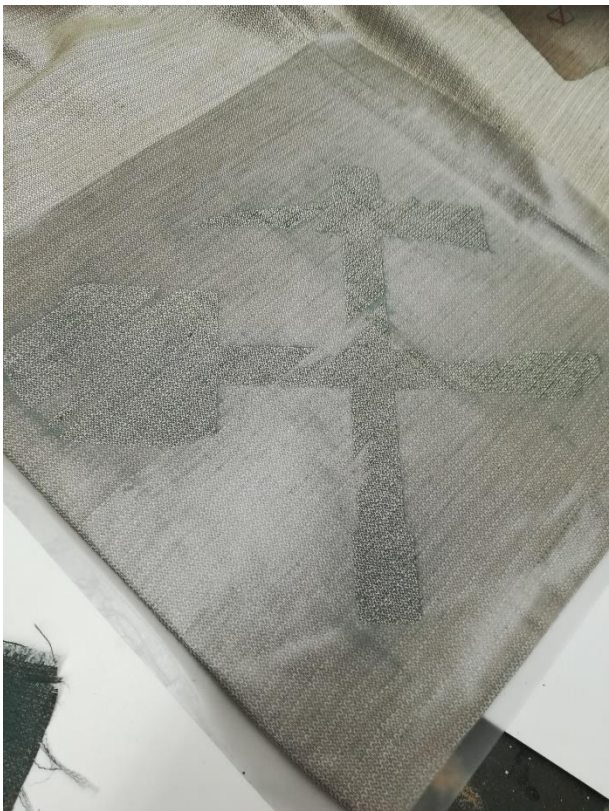
Step 5. The template is attached to the fabric. The imprint is made by a very thin layer of acrylic paint applied with a dry brush.
