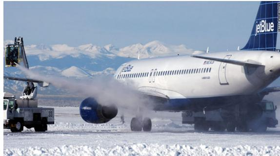
Figure 15.10: Chemical Anti-icing System
