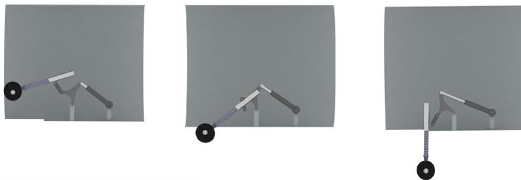
Figure 12.27: Nose Landing Gear Retraction Scheme
