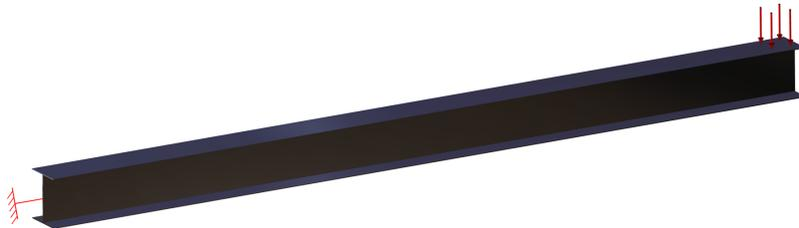
Figure 12.9: CATIA Structural Analysis Validation Model
